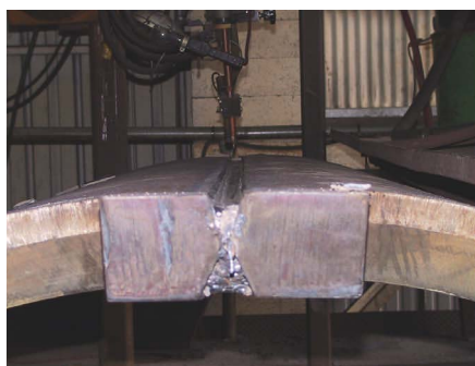
The cylinders required about 30 passes for the inside weld and about 30 passes for the outside weld.
